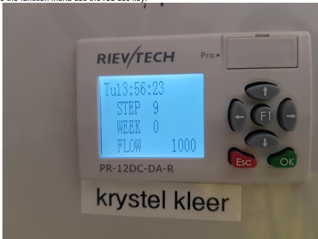
This also shows the 1000 litre emergency testing recorded on the PLC for Krystel Kloor STS.
